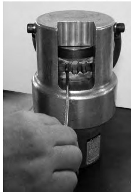
650 Portable Swager for use with all sizes of cable.
