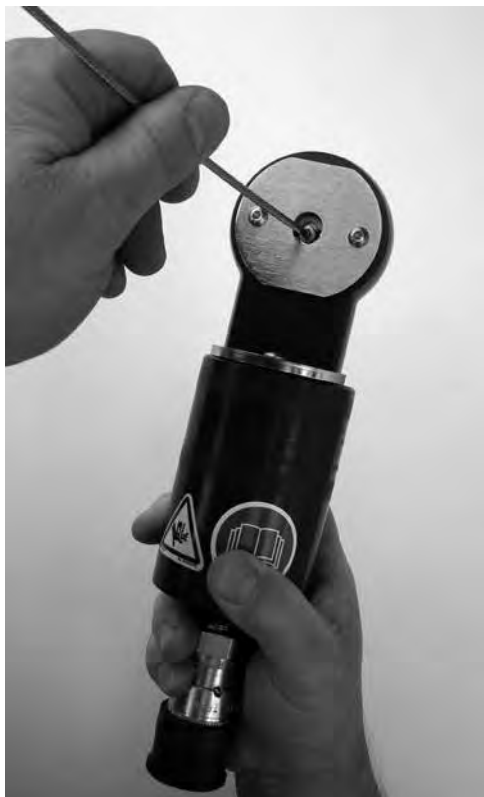
610 Portable Swager for use with 1/8" and 3/16" diameter cable.
