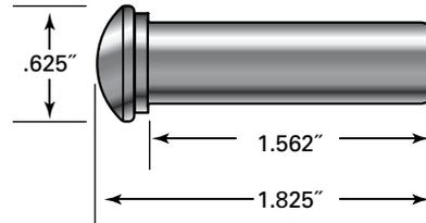
Pull-Lock™ stop-end fittings are made of type 316 stainless steel with the exception of internal components that are made of other types of stainless steel.
